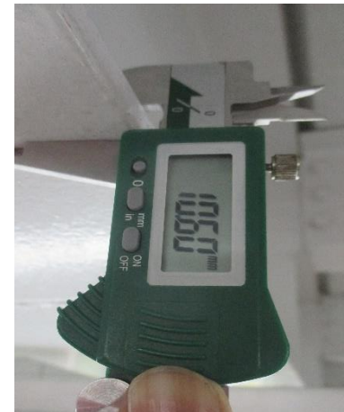
10 mm thickness of flange instead of 12 mm
