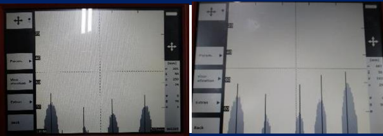
14nos. rebar was found on 3 rd floor
