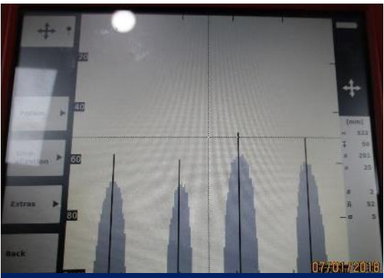
4 nos. rebar was found on long side
