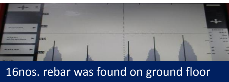
16nos. rebar was found on ground floor
