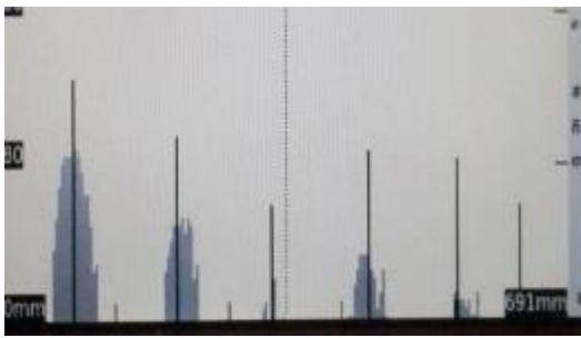
18 number of rebars were found by ferro scanning in C-2 type column
