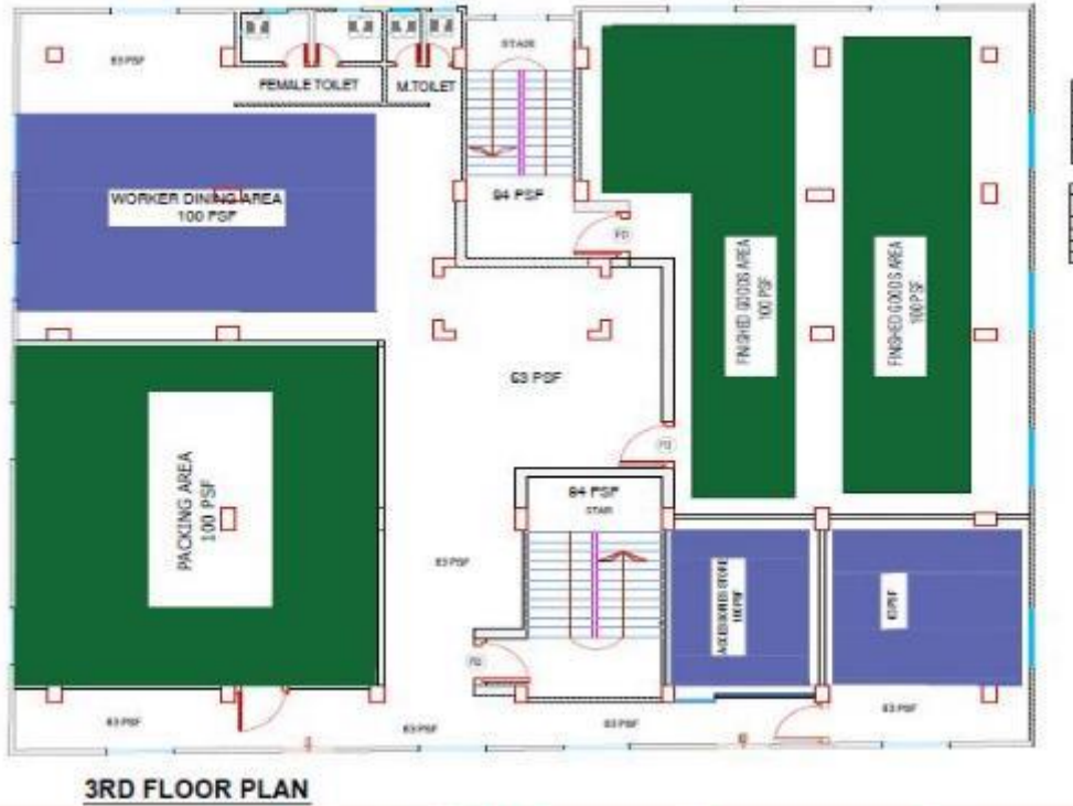
Loading on 3 rd floor packing section
