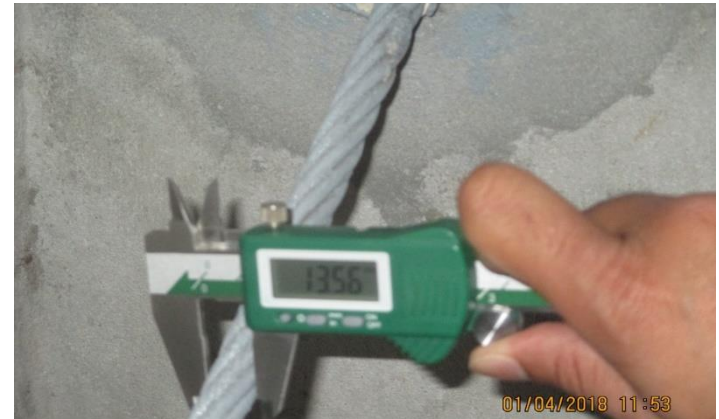
Dia of cable bracing
