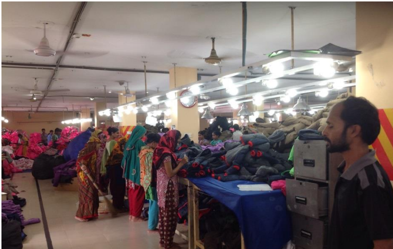
4 th Floor: Uncontrolled Finished Goods storage
